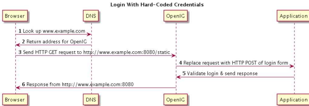
1. The browser host makes a DNS request for the IP address of the HTTP server host, `www.example.com`.
