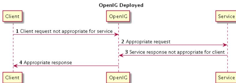
Clients then exchange with protected servers through OpenIG. This means that without touching either clients or servers, you can configure OpenIG to add new capabilities to existing services.
