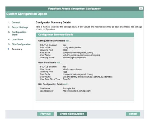
After you click Create Configuration in the summary screen, configuration proceeds, logging progress that you can read in your browser, and later, in the installation log. The process ends, and AM shows the Proceed to Login prompt.
